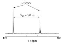
Fig. 5  $\,^{13}$ C NMR spectrum without  $^{1}$ H decoupling after 13.5 h irradiation for the same sample shown in Fig. 3.
