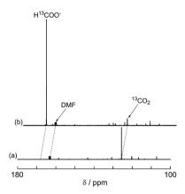
Fig. 3  $^{13}$ C{ $^{1}$ H} NMR spectra of the reaction solution before (a) and after (b) 13.5 h of irradiation: DMF- $d_7$ -TEOA (4:1 v/v) solution containing BI(OH)H (0.1 M), Ru<sub>2</sub>-Ru(CO) (0.5 mM), and  $^{13}$ CO<sub>2</sub> (569 mmHg) was irradiated at >420 nm using a xenon lamp.
