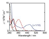
Fig. 1 UV-vis absorption spectra of BIH (black solid line), BI $^+$  (black broken line), BI(OH)H (red solid line), BI(O $^-$ ) $^+$  (red broken line), and Ru<sub>2</sub>-Ru(CO) (blue line, 1/10 intensity) in DMF-TEOA (4:1 v/v).
