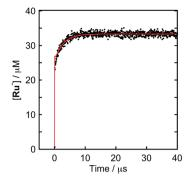
Fig. 8 Formation of Ru $^-$ : (a) DMF $^-$ TEOA (5 : 1 v/v) solution containing Ru (0.3 mM) and Bl(OH)H (0.1 M) was irradiated at  $\lambda_{\rm ex}=532$  nm with a Nd:YAG pulse laser under degassed conditions at room temperature. The red line shows the fitting results (ESI $^+$ ).
