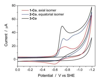
Fig. 4 Aqueous cyclic voltammetry of catalysts **1-Co** (red), **2-Co** (blue), and **3-Co** (black) in 1 M pH 7 KPBS at glassy carbon electrode. Catalyst concentration is 1 mM and scan rate = 100 mV s $^{-1}$ . Background is shown as a dotted gray line.
