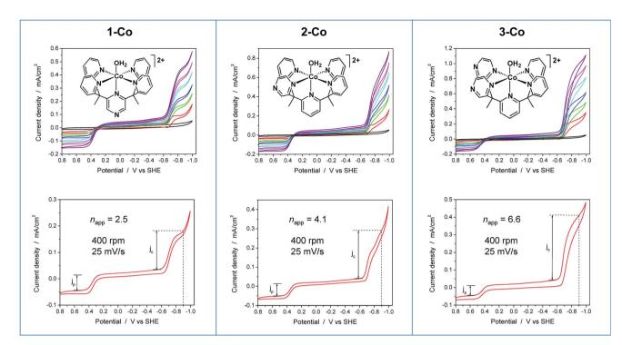
Fig. 6 RDEV of the series of cobalt catalysts. *Panels*: axial isomer **1-Co**,  $[(ax-PY4PZMe_2)Co(OH_2)]^{2+}$ ; equatorial isomer **2-Co**,  $[(eq-PY4PZMe_2)Co(OH_2)]^{2+}$ ; and catalyst **3-Co**,  $[(PY3PZ2Me_2)Co(OH_2)]^{2+}$ . *Top*: rotation rates of 100–3600 rpm; *bottom*: apparent  $n_{app}$  based on 1e<sup>-</sup> Co(III/III) couple at 400 rpm. *Conditions*: 0.3 mM catalyst, 0.1 M pH 7 KPBS, 0.1 M KNO<sub>3</sub>, 25 mV s<sup>-1</sup> scan rate, glassy carbon electrode (3 mm dia).
