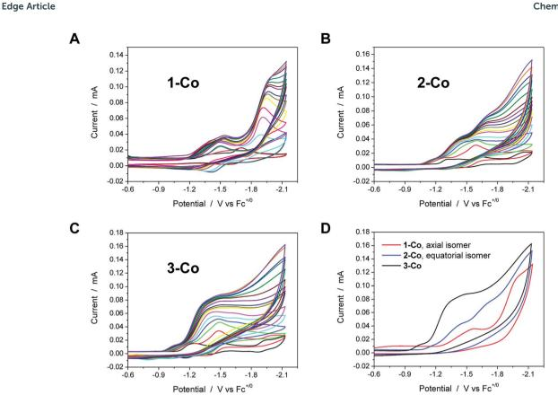
Fig. 3 Cyclic voltammetry of catalysts (1 mM) in acetonitrile with various concentrations of chloroacetic acid (up to 20 equivalents, 20 mM). A, B, and C. Catalysts **1-Co**, **2-Co**, and **3-Co**, respectively. The CV in black in these three graphs is the indicated catalyst in the absence of acid. D. Comparison of CVs for each catalyst, **1-Co** (red), **2-Co** (blue), and **3-Co** (black), with 20 eq. of chloroacetic acid. Scan rate =  $100 \text{ mV s}^{-1}$ ; 3 mm dia. glassy carbon.
