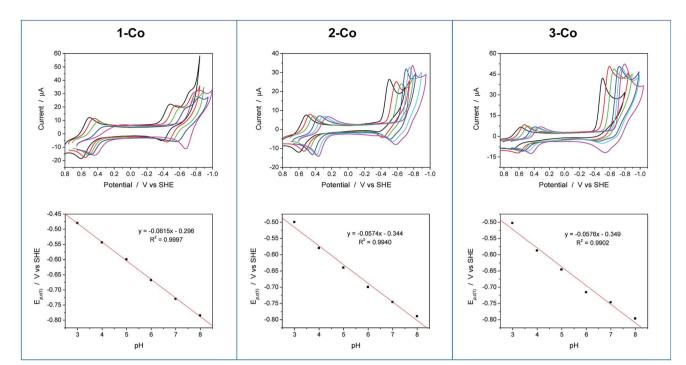
Fig. 5 Cyclic voltammograms as a function of pH and plots of the first reductive peak potential ( $E_{p,c(1)}$ ) vs. pH for **1-Co**, **2-Co**, and **3-Co**. Conditions: 0.9 mM catalyst, 0.03 M buffer, 0.1 M KNO<sub>3</sub>, 100 mV s<sup>-1</sup> scan rate, glassy carbon electrode (3 mm dia). Note: CV at pH 7 is omitted for clarity in series of CVs for **1-Co**. Legend: pH 3 (black), pH 4 (red), pH 5 (green), pH 6 (blue), pH 7 (cyan), pH 8 (magenta).
