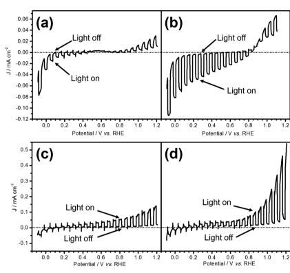
Fig. 1 Potential-current curves of (a) LTC/Au, (b) Pt/LTC/Au, (c) LTC/Ti, and (d) CoPi/LTC/Ti electrodes under visible light ( $\lambda$  > 420 nm) irradiation. The reference and counter electrodes used were an Ag/AgCl electrode and Pt wire, respectively. The potential was scanned in the positive direction.
