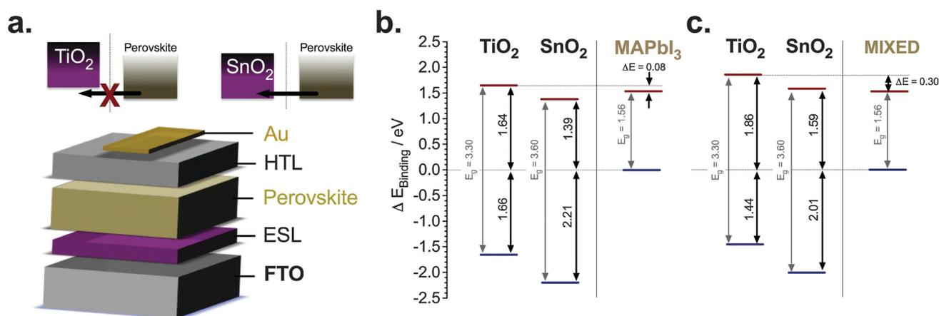
Fig. 1 Energy level diagrams and electron injection characteristics of SnO<sub>2</sub> and TiO<sub>2</sub>-based planar PSCs. (a) Schematic conduction band diagram of the perovskite films and the electron selective layers, TiO<sub>2</sub> and SnO<sub>2</sub> for (b) MAPbI<sub>3</sub> and (c) (FAPbI<sub>3</sub>)<sub>0.85</sub>(MAPbBr<sub>3</sub>)<sub>0.15</sub>, labeled as 'mixed'.
