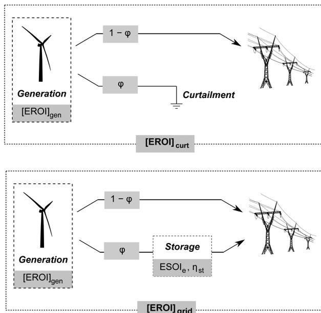
Fig. 5 A generating facility with  $[EROI]_{gen}$  may experience curtailment, resulting in an overall EROI of  $[EROI]_{curt}$ . Alternatively, the overgeneration may be routed through a storage facility, resulting in an overall EROI of  $[EROI]_{grid}$ .
