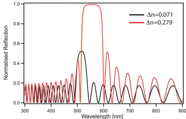
**Fig. 9** Refractive index dependence of one-dimensional stacks. The black line shows the calculated spectrum of a multilayer stack composed of 40 alternating 70 nm thick PS and PI layers (typical values for block copolymer based multilayers) obtained by the transfer matrix method. The red line corresponds to a multilayer stack with the same layer dimensions, where the PS layers are replaced by guanine.
