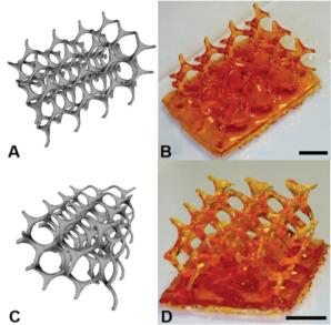
Fig. 2 3D CAD model of the modified (10,3)-a network used in this study (A and C). Fabricated (10.3)-a structure on a 400 µm baseplate to provide a favourable surface to build from and structural integrity (B and D). Scale bars are 2.5 mm.
