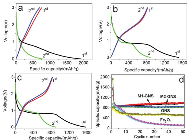
**Fig. 9** The initial two charge/discharge curves of (a) original GNS, (b) M1-GNS and (c) M2-GNS, and (d) cycling performance of M1-GNS, M2-GNS, GNS, and Fe<sub>3</sub>O<sub>4</sub> nanoparticles at the current density of 50 mA g<sup>-1</sup>.
