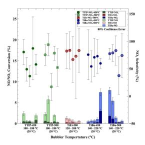
Fig. 5 Photocatalytic  $NO/NO_x$  conversion (bar chart) and  $NO_2$  selectivity (scatter chart) of samples grown at differing bubbler temperatures for a fixed synthesis time of 3 min (green-TTIP, red-TiEt, and blue-TiBu); the range of temperatures specified represent the range of bubbler temperatures studied from left to right in the bar chart, with temperatures in brackets representing the temperature intervals between each bar.
