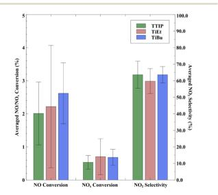
Fig. 7 The effect of the precursor type on average photocatalytic  $NO_x$  activity seen across the 58 samples produced herein (green-TTIP = 22 samples; red-TiEt = 14 samples; blue-TiBu = 22 samples). Error bars represent 80% confidence intervals.
