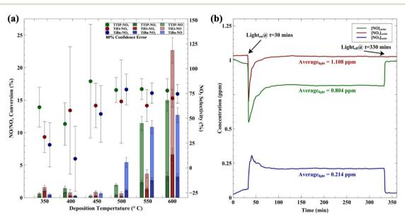
Fig. 3 (a) Photocatalytic NO/NO<sub>x</sub> conversion (bar chart) and NO<sub>2</sub> selectivity (scatter chart) of samples grown with differing deposition temperature (green-TTIP, red-TiEt, and blue-TiBu, from sample 001 to sample 012). (b) Photocatalytic  $NO_x$  measurement of sample 012\_TiEt\_600\_160\_3 measured under near-ISO test conditions (red-NO<sub>2</sub>, blue-NO<sub>2</sub>, and green-NO).
