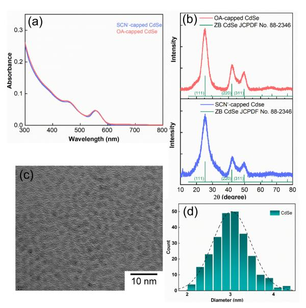
Fig. 1 (a) UV-vis absorption spectra of oleate-capped CdSe QD colloidal solution in hexane and thiocyanate SCN<sup>-</sup>-capped CdSe QD colloidal solution in DMF. (b) Diffraction patterns of QDs before and after ligand exchange revealing identical crystallinity. (c) HRTEM image of CdSe QDs before ligand exchange. (d) Particle size distributions with peaks at around ~3 nm are obtained from the HRTEM analysis of CdSe QDs.
