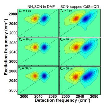
Fig. 3 2D IR spectra of NH<sub>4</sub>SCN (left column) and CdSe-SCN (right column) in DMF at three different waiting times ( $T_{\rm w}$ ).  $T_{\rm w}$  increases from the top to the bottom along each column.
