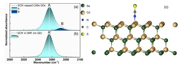
Fig. 2 (a) The FTIR spectrum of the  $C \equiv N$  stretching for SCN<sup>-</sup>-capped CdSe QD colloidal solution in DMF shows two overlapping transitions (A and B). (b) The FTIR spectrum of the  $C \equiv N$  stretching for SCN<sup>-</sup> in the absence of QDs shows a single symmetric peak (A'). (c) The optimized slab structure of the nitrogen terminated SCN<sup>-</sup>-capped (111) facet of the CdSe crystal.
