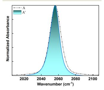
Fig. 5 The C≡N stretching peak of free SCN<sup>-</sup> in the absence of CdSe QDs (peak A') has been overlaid with the Gaussian fit of the peak at 2056 cm<sup>-1</sup> in the presence of QDs (peak A). The two spectra overlap well on the low-frequency side. In the presence of QDs, the Gaussian fit shows a broadening on the high-frequency side.
