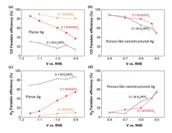
Fig. 1 Faradaic efficiencies for CO and  $H_2$  on flat Ag foil (a) (c) and porous-like nanostructured Ag (b) (d) at various potentials in 0.1 M  $K_2HPO_4$ , 0.1 M  $KHCO_3$  or 0.1 M  $KClO_4$  (all electrolytes were saturated with  $CO_2$ ), respectively. This figure has been reproduced from ref. 47 with permission from John Wiley and Sons, copyright 2016.
