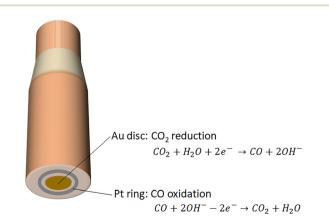
Fig. 3 Schematic illustration of rotating ring disc electrode. Electrocatalytic CO2 reduction to CO takes place on Au disc electrode, and subsequently oxidation of CO into CO2 occurs on Pt ring electrode.
