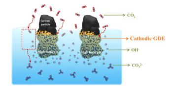
Fig. 4 Schematic illustration of  $CO_2$  capture at the cathodic GDE/catholyte interface in the form of carbonate via the neutralization reaction with  $OH^-$  during high-rate  $CO_2$  reduction. This Figure has been adapted from ref. 41 with permission from Royal Society of Chemistry, copyright 2022.
