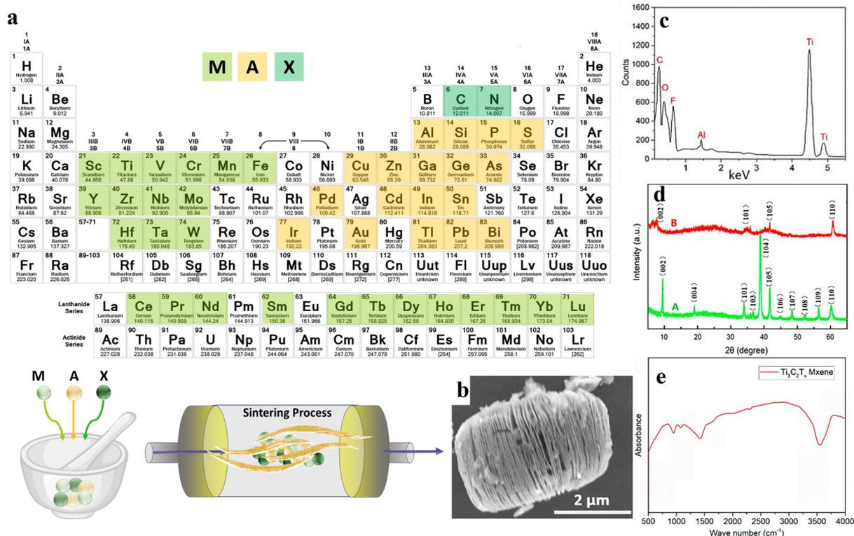
Fig. 3 The structure and synthesis of MXene nanosheets: (a) schematic illustration of the MXene structure and synthesis procedure. (b) SEM, (c) EDX, (d) XRD, and (e) FTIR results of  $\text{Ti}_3\text{AlC}_2$  and  $\text{Ti}_3\text{C}_2\text{T}_x$  powders. Reproduced from ref. 61 with permission from MDPI, Copyright 2020.
