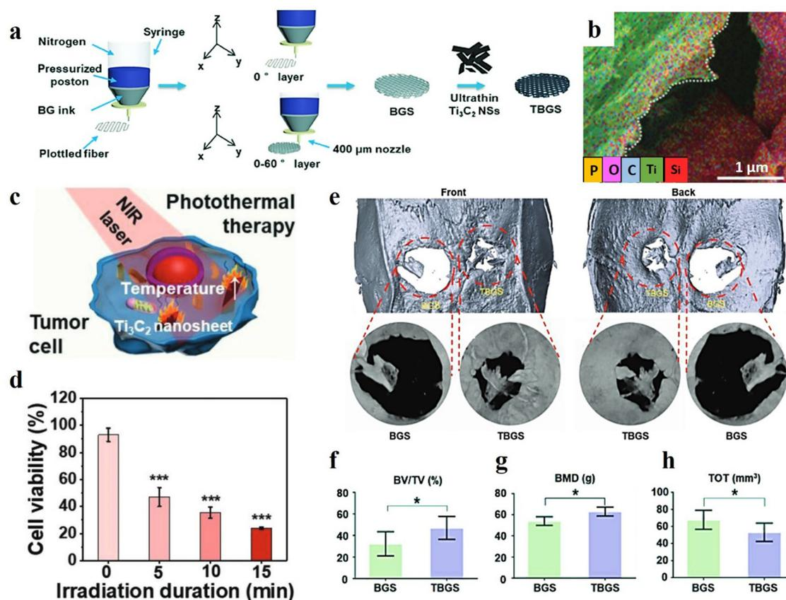
Fig. 5 Characteristics of a 3D-printed  $\text{Ti}_3\text{C}_2$ /bioactive glass bone scaffold; (a) schematic design of the synthesis methods, (b) EDS mapping, (c) and (d) schematic illustration of the photothermal therapy and its outcome, (e) evaluating the 3D reconstruction of the tissue after 24 weeks implantation of the composite tissues, and the value of (f) BV/TV, (g) BMD, and (h) TOT in newborn osseous tissues. Reproduced from ref. 18 with permission from Wiley, Copyright 2020.
