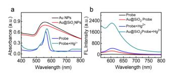
Fig. 2 (a) UV-vis spectra for 0.5 μM of the free fluorescent probe, Au@SiO $_2$  NPs, free fluorescent probe and fluorophore-labeled Au@SiO $_2$  probe with the addition of Hg $^{2+}$ . (b) Fluorescence spectra of the free probe, fluorophore-labeled Au@SiO $_2$  probe, and corresponding changes in fluorescence intensity after the addition of Hg $^{2+}$ . The concentration of the probe and Hg $^{2+}$  are all 0.5 μM.
