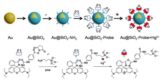
Scheme 1 Schematic illustration of the preparation flow for the fluorophore-labeled Au@SiO<sub>2</sub> NP probe and its detection mechanism for Hq<sup>2+</sup> ions.
