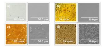
Fig. 7 Magnified (9x zoom) photos (left) and SEM images (right) to show surface features of X-poly(siloxane-r-S) (X = wt% S); X = (a) 0 (b) 5 (c) 10 (d) 15
