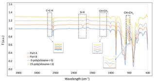
Fig. 4 Top: FT-IR spectra of (a) 10-poly(siloxane-r-S) after reacting with sulfur for 20 min (blue), 50 min (orange), 80 min (grey) and after solidification (yellow), and bottom: part A (blue), part B (orange), and 0poly(siloxane-r-S) after stirring for 2 h (grey) and 15-poly(siloxane-r-S) after solidification at 180 °C (yellow).
