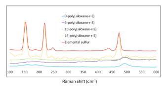
Fig. 6 Raman spectra of X-poly(siloxane-r-S) (X = wt% S); X = 0 (blue), 5 (purple), 10 (green), 15 (yellow), and S<sub>8</sub> (red).
