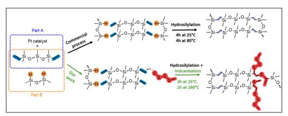
Fig. 2 Commercial synthesis (top route) of polysiloxane from the part A and part B moulding kits and our modified synthesis (bottom route) using S8 to generate X-poly(siloxane-r-S) (X = wt% S) with thermally repairable properties.
