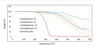
Fig. 8 Comparative TGA thermograms of X-poly(siloxane-r-S) (X = wt%S); X = 0 (blue), 5 (purple), 10 (green), 15 (yellow), and  $S_8$  (red).
