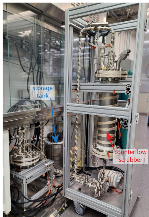
Fig. 2 Molten hydroxide (NaOH-KOH eutectic) showing interior before insulation. The external salt storage tank is shown on the left. This figure was modified from the original by McFarlane et al. 89 and reprinted with permission.
