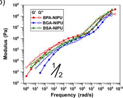
Fig. 5 Frequency-dependent storage (G') and loss (G") moduli for (a) unsubstituted bridging carbon- and (b) dimethyl-substituted bridging carbonbased NIPUs. The master curves were constructed using time-temperature superposition and reported at 150 °C. Lines indicate typical power-law scalings of G' (slope of 2) and G'' (slope of 1)
