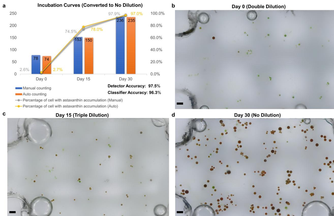
**Fig. 5** Monitoring the accumulation of astaxanthin in *Haematococcus Pluvialis*. a) Culture experiment data and comparison graph of manual and AIMP obtained statistics. Example images of a single observation chamber at b) day 0 (samples are diluted twofold before adding to the chip), c) day 15 (samples are tripled diluted before adding to the chip), and d) day 30 (samples are not diluted). Scale bars are 200  $\mu\text{m}$ .
