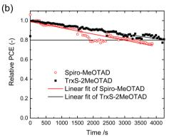
Fig. 8 Operational stability of TrxS-2MeOTAD compared with spiro-MeOTAD (ISOS-L-1). The cells were held at a constant voltage, at the initial maximum power point and the current density was recorded under constant illumination at 1 sun until the current (and calculated efficiency) dropped to 80% of the initial value. (a) From t = 0 s to t = 300 s. (b) From t = 0 to t = 4000 s
