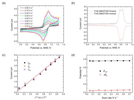
Fig. 4 (a) Cyclic voltammogram of TrxS-2MeOTAD at different scan rates ranging from  $0.05 \text{ V s}^{-1}$  to  $0.70 \text{ V s}^{-1}$ . (b) Square wave voltammogram of TrxS-2MeOTAD at a scan rate of 0.05 V s<sup>-1</sup>. (c)  $I_{pa}$ ,  $I_{pc}$  and  $I_{1/2}$  versus square-root of the scan rate  $v^{0.5}$  derived from (a);  $R^2 = 0.992$  for the linear fitting of  $I_{1/2}$ . (d)  $E_{1/2}$  and  $\Delta E_{\rm p}$  versus scan rate, derived from (a)
