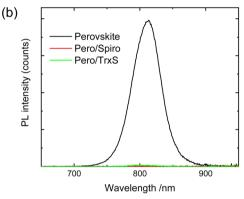
Fig. 6 (a)  $J^{0.5}-V$  curves used to derive the hole mobility from SCLC measurements. (b) Steady-state photoluminescence spectra of spiro-MeOTAD/perovskite and TrxS-2MeOTAD/perovskite films.
