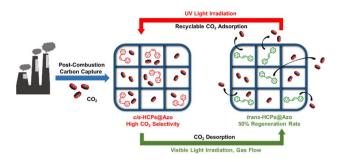
Fig. 1 Our approach of exploiting photo-isomerisation of azobenzene molecules embedded in pores of HCPs to drive adsorption (upon UV irradiation) and desorption (vis-irradiation) of  $CO_2$  to enable low-energy, low-cost carbon capture.
