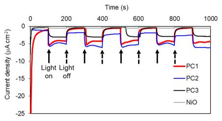
Fig. 4 Representative example of photocurrent in 0.1 M pH 5 acetate buffer under chopped light illumination for photoelectrocatalysis experiments of NiO films sensitized with photocatalysts. The applied bias was -0.2 V vs. Ag/AgCl. NiO, PC1|NiO and PC3|NiO are saturated with CO2, PC2|NiO is saturated with Ar.
