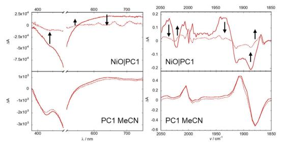
Fig. 3 UV-visible transient absorption spectra (left) and time resolved infrared spectra (right) for PC1, 1 ps (solid line) and 1 ns (dotted line) following excitation at 500 nm in acetonitrile (bottom) and on a NiO thin film (top). The transient features at 1 ns spectrum for NiO/PC1 are imprints of the probe spectrum.
