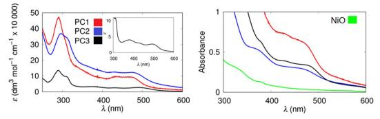
Fig. 2 Left panel: steady-state absorption spectra of the photocatalysts in acetonitrile. Right panel: absorption spectra of the same systems when adhered to NiO electrodes following dye-bath deposition.
