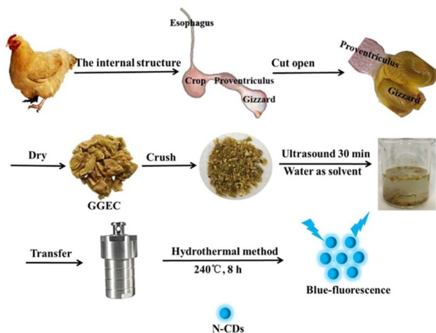
Fig. 6 A systematic diagram of N-CDs derived from GGEC by the HT method. Reprinted from ref. 216, Copyright (2021), with permission from Elsevier.
