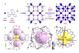
Fig. 3 Porous structure of ZNU-6. (a)–(c) Exquisite control of pore size/shape and pore chemistry in ZNU-6 from pillared (3,4)-connected pto network to  ${\rm GeF_6}^{2-}$  embedded ith-d topology framework; (d) overview of ZNU-6 structure with cage-like pores and interlaced channels. (e) Structure and size of the cage-like pore. (f) Structure and size of the interlaced channel connecting four cages.<sup>42</sup>
