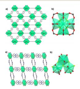
Fig. 4 On top: crystal structure of Ho-UiO-66 MOF. (a) Extended view along the a direction. (b) Holmium hexacluster containing  $\mu_3$ -F bridging groups. Reprinted with permission from ref. 44. Copyright 2021 American Chemical Society. On the bottom: crystal structure of Ho-4,4'-BPDC MOF. (a) Extended view along the a direction. (b) Holmium tricluster containing one  $\mu_3$ -F group. Reprinted with permission from ref. 44. Copyright 2021 American Chemical Society.
