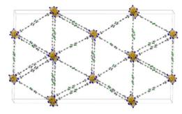
Fig. 13 Crystal structure of Fe-PF4 MOF extended view along (1 1 1) *hkl* direction. Colour code: iron polyhedra orange, carbon grey, nitrogen blue, fluorine green and hydrogen white.<sup>68</sup>
