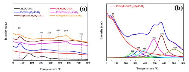
Fig. 3 CO<sub>2</sub>-TPD profiles of (a) Ni-based Al<sub>2</sub>O<sub>3</sub>-CeO<sub>2</sub>. (b) The fine structure of the Pt/MgFe/Ni/Al<sub>2</sub>O<sub>3</sub>-CeO<sub>2</sub> composite catalysts.
