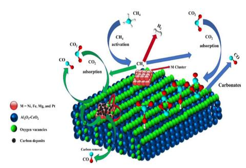
Fig. 7 Schematic representation of a plausible reaction over the (M = Pt, Mg, and Fe) doped Ni/Al<sub>2</sub>O<sub>3</sub>-CeO<sub>3</sub> catalysts.
