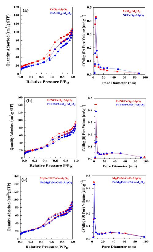
Fig. 5 ((a-c), left side)  $N_2$  physisorption isotherms and ((a-c), right side) BJH pore size distribution of Ni-based  $Al_2O_3$ -Ce $O_2$  composite catalysts.
