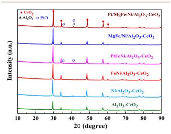
Fig. 1 XRD patterns of Ni-based Al<sub>2</sub>O<sub>3</sub>-CeO<sub>2</sub> composite catalysts.
