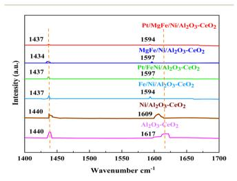
Fig. 4 Pyridine IR spectra of Ni-based  $Al_2O_3$ -Ce $O_2$  composite catalysts.
