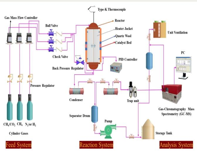
Scheme 1 Schematic diagram of the experimental setup for the dry reforming of methane.
