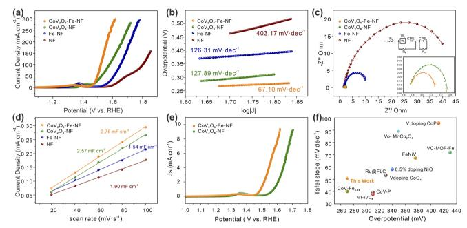
Fig. 4 The OER performance of the electrocatalysts in 1.0 M KOH. (a) LSV curves, (b) Tafel slopes, (c) Nyquist curves, (d) double layer capacitances, (e) ECSA normalized LSV curves and (f) comparison of  $COV_2O_6$ -Fe-NF with other reported similar OER electrocatalysts in alkaline media.
