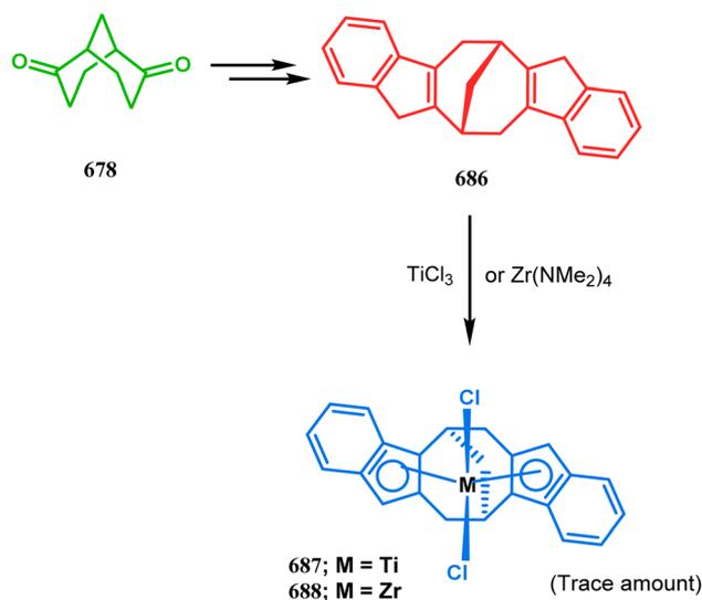
Scheme 155 Synthesis of titanium and zirconium complex.
