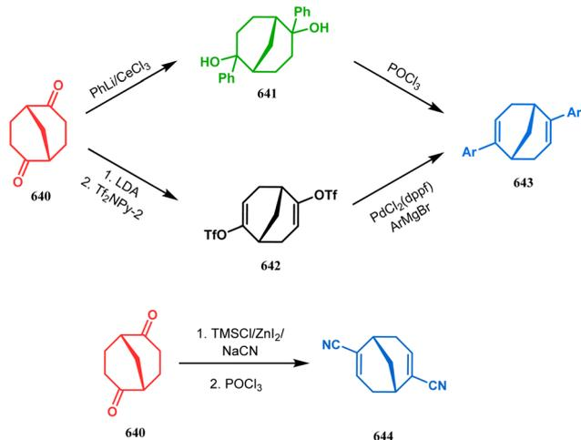
Scheme 145 (a) Synthesis of bicyclo[3.3.1]nonane-based chiral diene ligands (b) synthesis of dicyanobicyclo[3.3.1]nonane.
