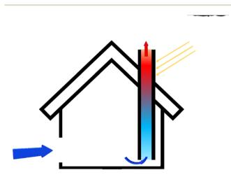
Fig. 11 Schematic of solar chimney
