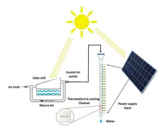
Fig. 9 Schematic of TEC-based distillation system.
