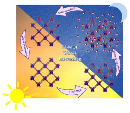
Fig. 21 Steps of atmospheric water harvesting used desiccants.
