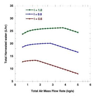
Fig. 6 Total harvested water volume flow rate (L  $h^{-1}$ ) as a function of total air mass flow rate (kg s $^{-1}$ ) for different solar radiation intensity (kW  $m^{-2}$ ). Reproduced from ref. 40 with permission from International Journal of Energy Research.
