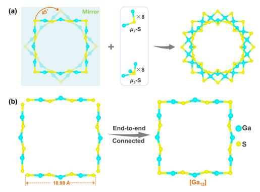
Fig. 2 (a) Mirror symmetric two [Ga<sub>12</sub>] folded quasi-ideal square (coordinated CPA is omitted) linked together through 8  $\mu_2$ -S<sup>2-</sup> and 8  $\mu_3$ -S<sup>2-</sup> by twisting ~45° to form the wheel-shaped molecular ring and (b) a [Ga<sub>12</sub>] unit constructed by 4 1D polymeric chains of 3 Ga<sup>3+</sup> ions and 4 adjacent bridged  $\mu_2$ - $S^{2-}$ .
