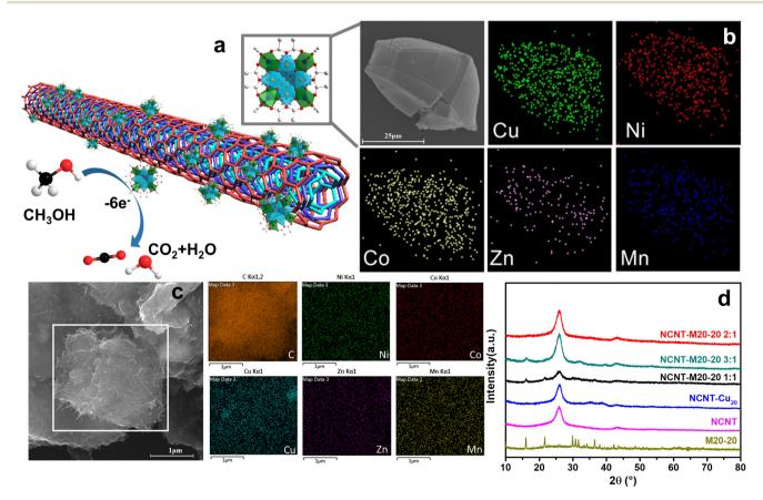
Fig. 2 Structural characterizations of the NCNT-M20-20 composite. (a) Graphic illustration of NCNT-M20-20 2:1 in the MOR process, with the structure of M20-20 shown as a ball-stick model. (b) Morphology of M20-20 and mapping information of the selected area. (c) Morphology of NCNT-M20-20 2:1 and EDS results. (d) Powder XRD of a series of materials.
