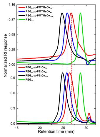
**Fig. 5** SEC chromatograms of PEG, PEG-*b*-PEtOx, and PEG-*b*-PMTMeOx with different degrees of polymerizations.
