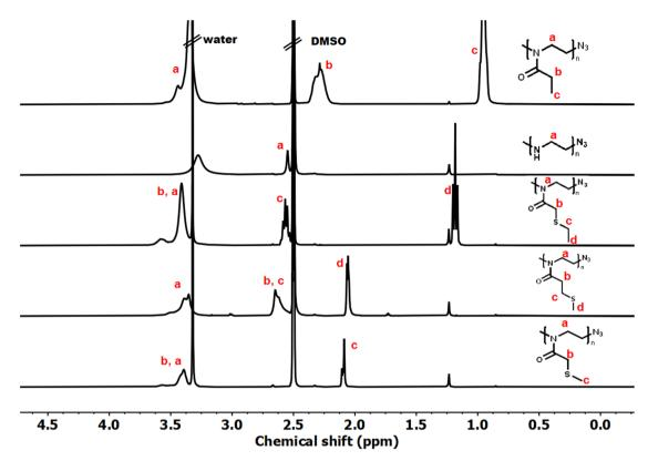
Fig. 1 Representative <sup>1</sup>H NMR spectra of PEtOx, PEI, PMTMeOx, PMTEtOx, and PETMeOx in DMSO-d<sub>6</sub>.
