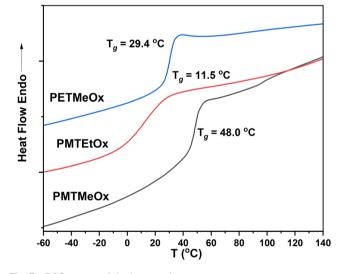
Fig. 3 DSC curves of the homopolymers.
