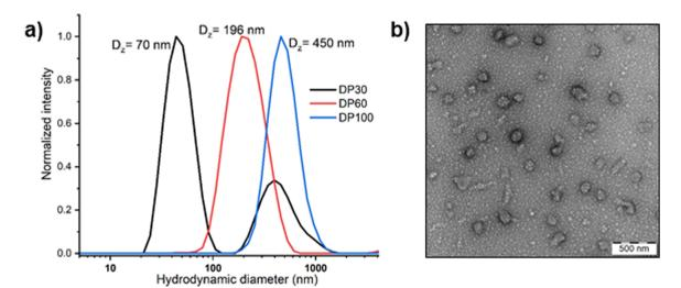
Fig. 6 (a) Hydrodynamic size distributions of  $PEG_{45}$ -PMTMeOx<sub>x</sub> micelles of different PMTMeOx DP measured by DLS in water ( $c_{pol} = 1 \text{ mg mL}^{-1}$ ) and (b) TEM image of  $PEG_{45}$ -b-PMTMeOx<sub>30</sub> nanoparticles.
