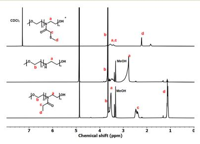
Fig. 4 <sup>1</sup>H NMR spectra of PEG-*b*-PMTMeOx in CDCl<sub>3</sub>; and PEG-*b*-PEI and PEG-*b*-PEtOx, in CD<sub>3</sub>OD (\*some –OH groups were transformed into their respective esters).
