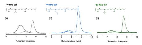
Fig. 4 SEC analysis of copolymers before (solid lines) and after hydrolytic degradation (dashed lines) under accelerated conditions. Light scattering signals of (a) <sup>1</sup>Pr-MAC-25T, (b) <sup>n</sup>Pr-MAC-25T and (c) <sup>t</sup>Bu-MAC-25T are depicted.
