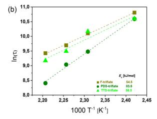
Fig. 5 (a) Normalized stress relaxation curves (obtained at 180 °C) of thiol-acrylate networks as a function of triphenylsulfonium salts with varying cations. Prior to the measurements the films were UV irradiated with a mercury emitter for 10 s ( $\lambda = 200-550$  nm, 20 mW cm<sup>-2</sup>). (b) Arrhenius plots derived from the measured relaxation times of catalysed thiol-acrylate networks.
