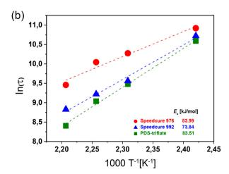
Fig. 3 (a) Normalized stress relaxation curves (obtained at 180 °C) of catalysed and non-catalysed thiol-acrylate networks as a function of triphenyl-sulfonium salts with varying counter anions. Prior to the measurements the films were UV irradiated with a mercury emitter for 10 s ( $\lambda$  = 200–550 nm, 20 mW cm<sup>-2</sup>). (b) Arrhenius plots derived from the measured relaxation times of catalysed thiol-acrylate networks.
