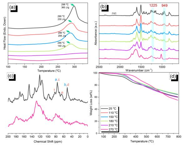
Fig. 6 (a) DSC, (b) FTIR spectral, (c) solid-state NMR spectral, and (d) TGA analyses of the TPA-DHTP-BZ POP after thermal ROP at various temperatures.
