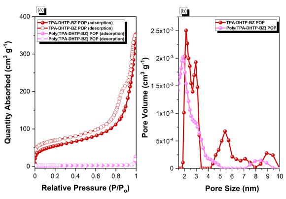
Fig. 7 (a) N₂ adsorption/desorption isotherms at 77 K and (b) pore size distributions of the TPA-DHTP-BZ POP and poly(TPA-DHTP-BZ) POP.
