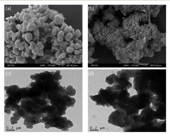
Fig. 8 SEM and TEM images of the TPA-DHTP-BZ POP (a and c) and poly(TPA-DHTP-BZ) POP (b and d).
