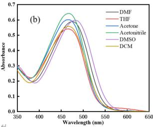
Fig. 1 (a) Absorption spectra of the chalcones ( $c = 1 \times 10^{-5}$  mol L<sup>-1</sup>). (b) TPA-2 absorption peaks in different solvents.
