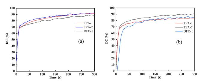
Fig. 3 Photopolymerization kinetics of the chalcones/lod/EDAB systems (chalcones: 0.1 wt%; Iod: 1.0 wt%; EDAB: 1.0 wt%, TMPTA as monomer) under different light sources (a) 365 nm LED, (b) 405 nm LED.
