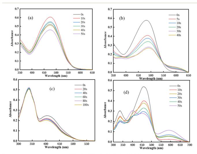
Fig. 4 Steady state UV degradation of chalcones: (a) TPA-1/lod; (b)TPA-2/lod; (c) DFO-1/lod; (d) DFO-2/lod.
