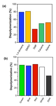
Fig. 2 Depolymerization conversion after 8 hours of PMMA-DTB with 100 ppm Eosin Y at 5 mM and 100 °C using (a) different solvents under green irradiation, and (b) different wavelength irradiation in 1,4-dioxane.
