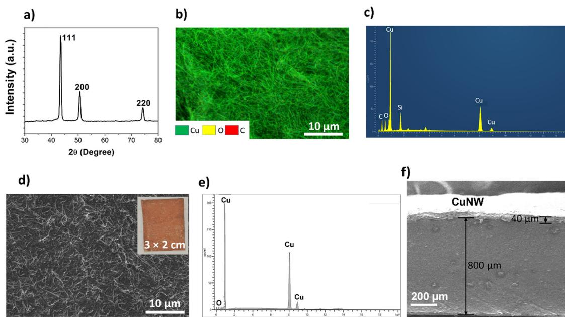
Fig. 2 (a) XRD pattern of the CuNWs, (b) SEM and elemental mapping of the as synthesized CuNWs, (c) EDS spectra of the CuNWs before lactic acid treatment, (d) SEM of the CuNW electrode layer after lactic acid treatment (inset-image of the electrode on adhesive tape), (e) corresponding EDS spectra and (f) cross-section SEM image of the TENG showing the Ecoflex and CuNW layer.
