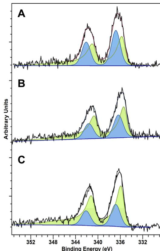
Fig. 1 XPS spectra of Pd(3d) regions of the as-prepared (A) 0.25%Pd–0.25%Sn/TiO<sub>2</sub>, (B) 0.25%Pd–0.25%Au/TiO<sub>2</sub> and (C) 0.5%Pd/TiO<sub>2</sub> catalysts. Key: Pd<sup>0</sup> (green) Pd<sup>2+</sup> (blue).
