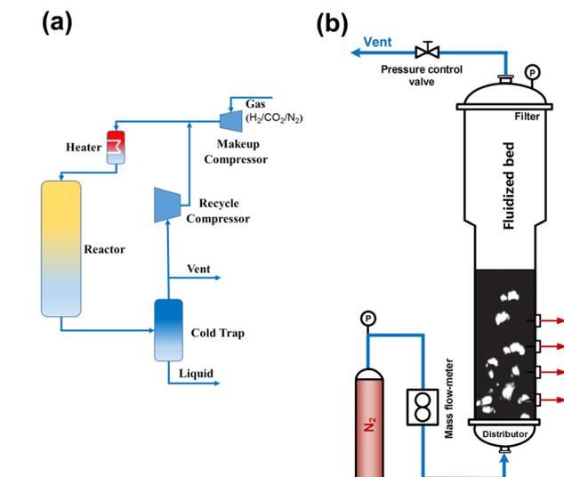
Fig. 14 (a) Schematic flow diagram of the pilot-scale fixed-bed reactor,<sup>49</sup> (b) schematic diagram of the cold-flow apparatus.<sup>110</sup> Reproduced from ref. 49 and 110 with the permission from Springer Nature and Wiley, copyright 2017 and 2022.
