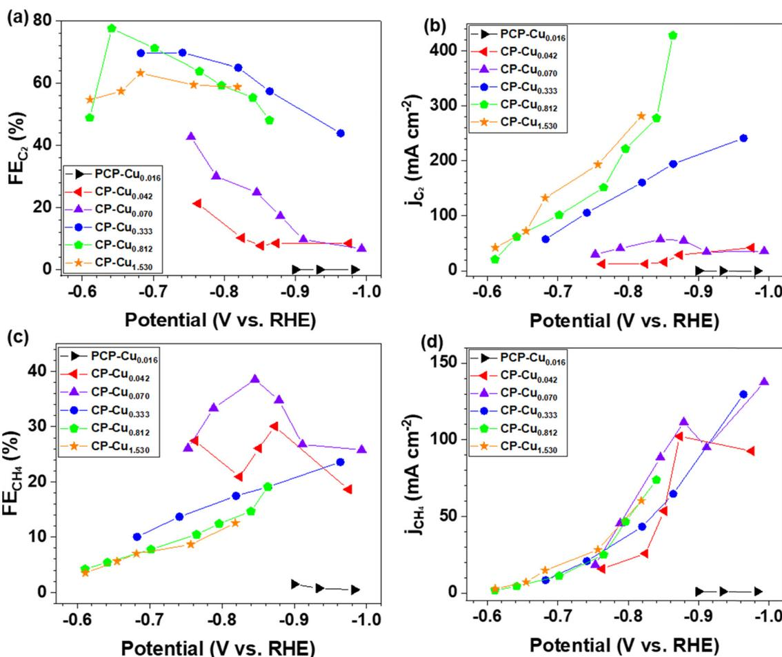
Fig. 2 (a) The partial current density and (b) FE of C<sub>2</sub> during the CORR as a function of the applied potential using CP-Cu electrodes with various Cu loadings. (c) The partial current density and (d) FE of CH<sub>4</sub> as a function of the applied potential using CP-Cu electrodes with various Cu loadings.
