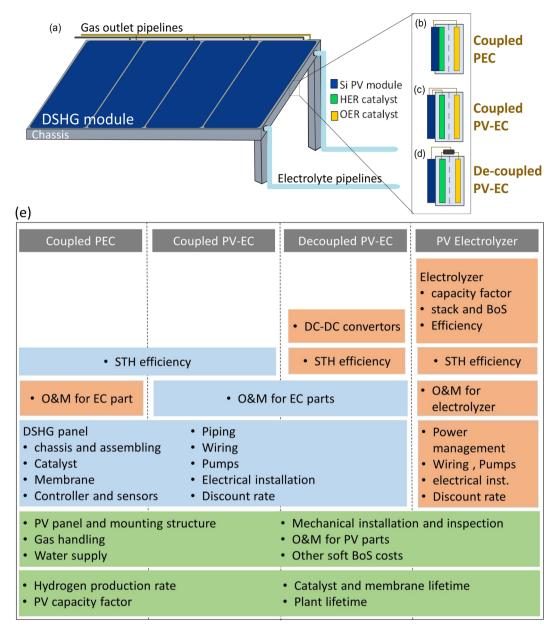
Fig. 1 Schematic of (a) direct solar hydrogen generation (DSHG) module. Different configurations analysed (b) coupled PEC, (c) coupled PV-EC and, (d) decoupled PV-EC DSHG. (e) Cost breakdowns for all three DSHG system configurations and off grid PV-Electrolyser. Operating conditions and component costs that are identical to all the four systems are shown in green. Costs common in two or more systems are shown in blue and orange shows the costs specific to each system
