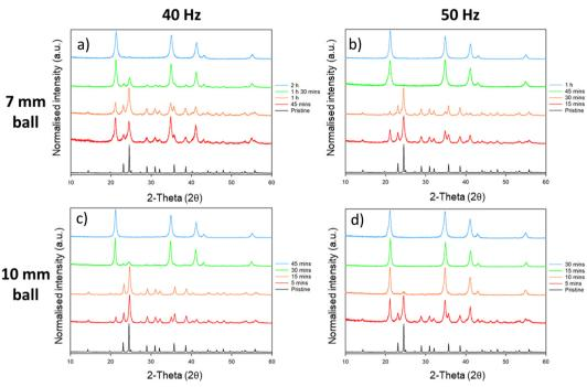
Fig. 6 Resulting PXRD patterns from the study of ball mill frequency, time and ball size on the milling of  $Li_2MoO_4$ . Patterns (a) and (b) made use of a 7 mm ball at 40 Hz and 50 Hz, respectively. Patterns (c) and (d) made use of a 10 mm ball at 40 Hz and 50 Hz respectively. The conversion rate was shown to significantly reduce with lower frequency or ball size. (Co  $K\alpha$ ). 50 mg of material was loaded into the pots in each case.
