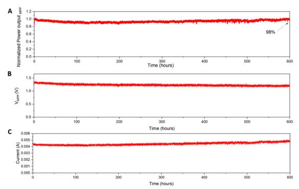
Fig. 5 Stability testing of encapsulated  $1 \, \text{cm}^2$  perovskite-Si tandem cells under continuous illumination (100 mW cm<sup>-2</sup>) at relative humidity of  $60 \pm 20\%$  at room temperature. Maximum power point tracking of (A) power output, (B) voltage ( $V_{\text{MPP}}$ ) at the maximum power point and (C) current to the starting value at the maximum power.
