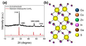
Fig. 1 Figure of (a) powder X-ray diffraction pattern of thin film (CoCuZn-Galn)S with reference to standard chalcopyrite (CulnS<sub>2</sub>, ICSD: 66865). (b) The crystal structure of HE chalcopyrite (a = b = 5.52, c = 11.13,  $\alpha$  =  $\beta$  =  $\gamma = 90^{\circ}$ ).
