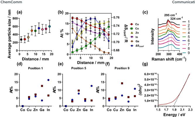
Fig. 3 (a) Particle size distribution analysis across the film of the SEM images (Fig. S8, ESI†). (b) SEM-EDX elemental analysis across the film. (c) Raman spectra obtained across the film (d)-(f) XPS (blue circles) vs. HAXPES (red squares) atomic abundance determined from (d) the initial 1-3 mm, (e) 9-11 mm and (f) 17-20 mm of the film. (g) Tauc plot of the UV-Vis spectra shown in Fig. S23 (ESI†).
