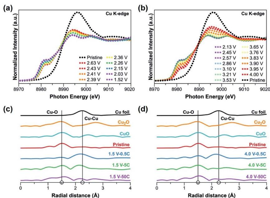
Fig. 4 XAS of  $[\text{CuL}(\text{Py})_2]_n$  electrodes: (a) and (b) *in situ* Cu K-edge XANES patterns during discharge and charge at  $20 \text{ mA g}^{-1}$  ( $\sim 0.08\text{C}$ ), respectively. (c) and (d) *Ex situ* Cu K-edge EXAFS patterns at three different rates (0.5C, 5C and 50C) at end of discharge (1.5 V) and end of charge (4.0 V), respectively (with Cu foil,  $\text{Cu}_2\text{O}$  and CuO as references).
