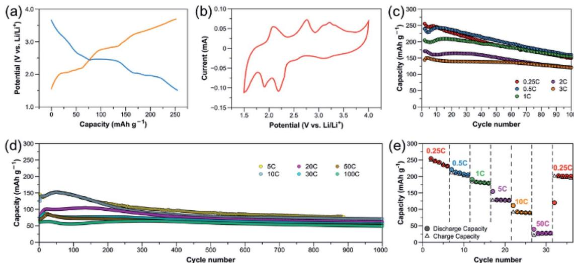
Fig. 2 Electrochemical properties of  $[\text{CuL}(\text{Py})_2]_n$  cathode: (a) discharge–charge profile at 0.25C ( $\sim 65 \text{ mA g}^{-1}$ ). (b) CV plot with a scan rate of  $0.5 \text{ mV s}^{-1}$ . (c) Capacity retention at rates of 0.25C to 3C ( $\sim 785 \text{ mA g}^{-1}$ ). (d) Capacity retention at rates of 5C ( $\sim 1308 \text{ mA g}^{-1}$ ) to 100C ( $\sim 26\,162 \text{ mA g}^{-1}$ ). (e) Rate capability at various current densities.
