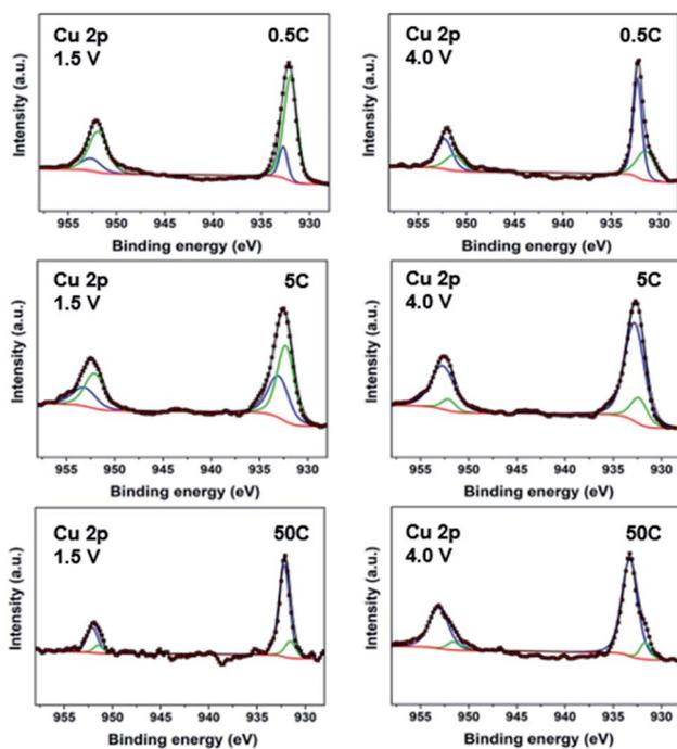
Fig. 3 Deconvolution of Cu  $2p_{3/2}$  and  $2p_{1/2}$  XPS spectra of  $[\text{CuL}(\text{Py})_2]_n$  electrodes at various rates. 0.5C (top), 5C (middle) and 50C (bottom) at end of discharge (1.5 V, left) and end of charge (4.0 V, right) (green: Cu(0); blue: Cu(I)).
