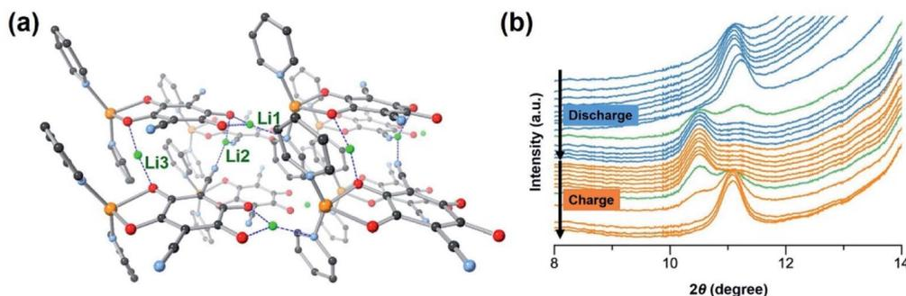
Fig. 5 (a) Computational simulation of lithiated CP  $[\text{CuL}(\text{Py})_2\text{Li}_3]_n$  showing the DFT optimized structure. Colours of atoms: orange:  $\text{Cu(I)}$ ; grey: C; red: O; cyan: N; green: Li; H is omitted for clarity. (b) *In situ* synchrotron PXRD patterns of CP electrode collected during the first discharge–charge cycle at current density of  $120 \text{ mA g}^{-1}$  at a voltage between 1.5 V and 4.0 V.
