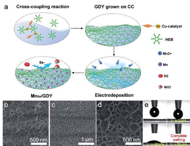
Fig. 1 (a) Schematic representation of the synthetic process of \text{Mn}_{\text{SA}}/\text{GDY} . (b) SEM image of GDY. (c and d) SEM images of \text{Mn}_{\text{SA}}/\text{GDY} at different scale bars. (e) Contact angle measurements of \text{Mn}_{\text{SA}}/\text{GDY} .
