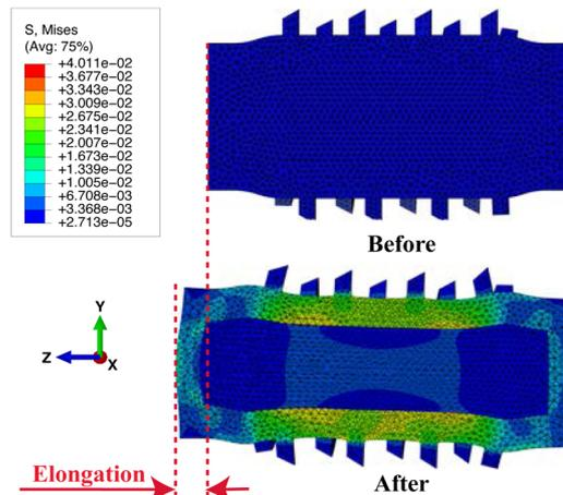
Fig. 7 Before and after the deformation of a 2 mm thickness segment with incompressible filling. The colour scale indicates Von Mises stress values.
