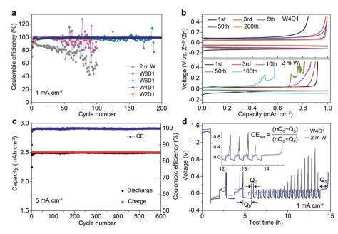
Fig. 3  $Zn^{2+}$  plating/stripping behaviors in H<sub>2</sub>O + DMC electrolytes. (a) Zn plating/stripping CE values of Zn/Ti cells in different electrolytes. (b) Typical voltage profiles of Zn/Ti cells in W4D1 and 2 m W at 1 mA cm<sup>-2</sup>. (c) Cycling stability and Zn plating/stripping CE of the Zn/Ti cell in W4D1 at 5 mA cm<sup>-2</sup>. (d) Evolution of voltage profiles of Zn/Ti cells in W4D1 and 2 m W electrolytes under a 'reservoir half-cell' method.
