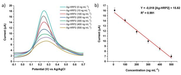
Fig. 6 a) DPV recorded with the Ab-PfHRP2/DHP/GE electrochemical immunosensor upon additions of Ag-PfHRP2 (10, 100, 200, 300, 400, and 500 ng mL<sup>-1</sup>), (b) calibration curve: Y = -0.018 [Ag-PfHRP2] + 15.82, with an  $R^2 = 0.991$ .
