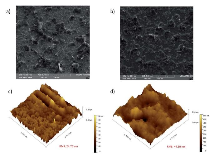
SEM and 3-dimensional AFM images: (a and c) DHP/GE surface, (b and d) Ab-PfHRP2/DHP/GE surface
