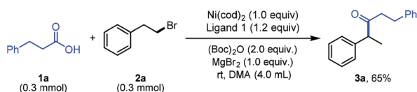
Scheme 2 Stoichiometric reaction without electric current.
