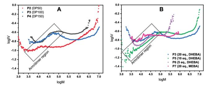
Fig. 2 Mark—Houwink (log IV vs. log M) plots for P2 (red), P3 (blue) and P4 (black) investigating the effect of arm degree of polymerisation (A), and for P3 (blue), P5 (green), P6 (purple), and P7 (pink) investigating the effect of cross-linker equivalents on formation of CCS polymers (B).
