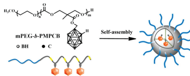
Scheme 1 Structure of the amphiphilic carborane-conjugated polycarbonate and self-assembly in water, adapted from ref. 20 with permission from the American Chemical Society, copyright 2016.
